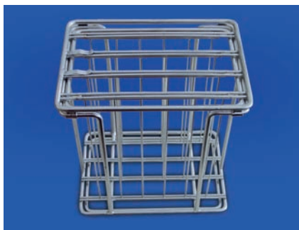
The workpiece holders were designed to hold 24 stents in a vertical position. The rods are held in place by the double rounds in the lid. (Photo: Metallform)
