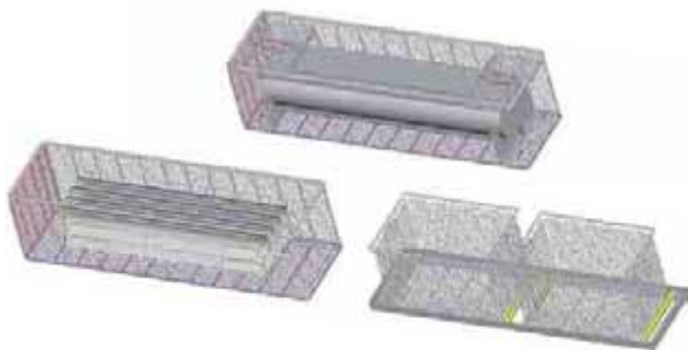
Customised basket with parts-specific holders for large parts and adapter frame for adapting standard MEFO-BOXes to the non-standard batch size (figure 1)
