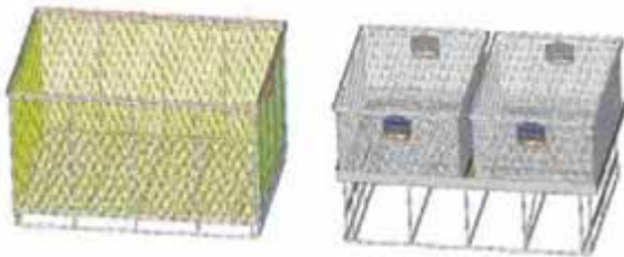
Customised basket for large parts and adapter frame for adapting standard MEFO-BOXes to the non-standard batch size.
